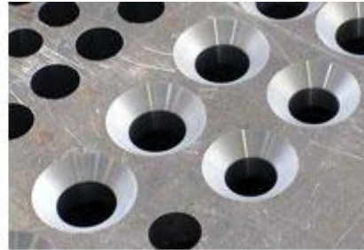
With Novator's orbital holemaking system, tools from Kennametal (left) reportedly can drill through stacks of metal and composite layers without delaminating the composite's fibers.
